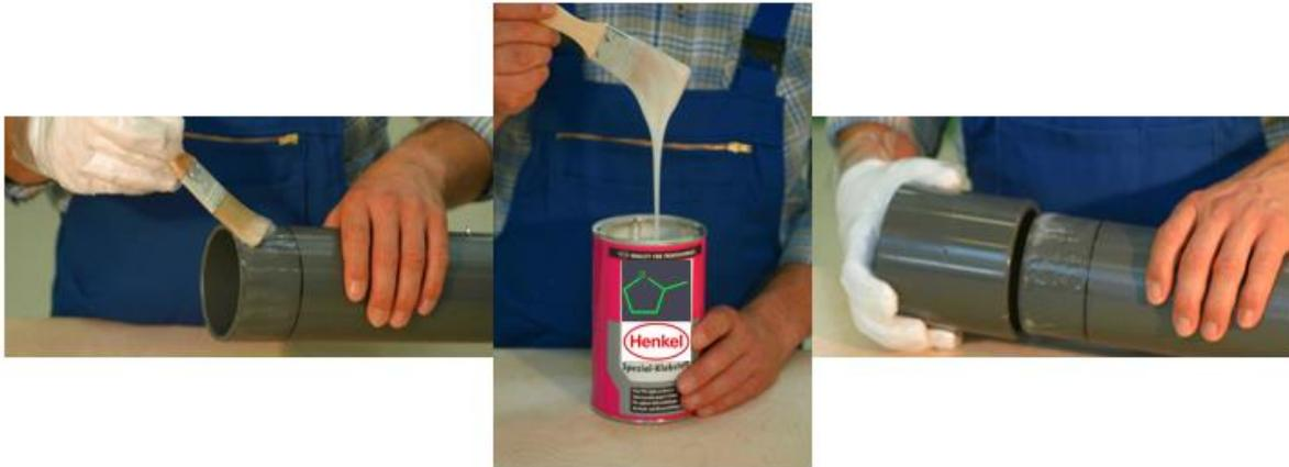
**Figure 1: Pipe adhesive prototype containing potentially green solvent MTHF.**
