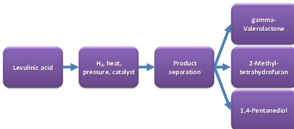
**Figure 1: Second part of the value chain demonstration: Hydrogenation of levulinic acid to high-value products and building blocks.**
